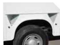
WHEEL CHOCK HOLDER - FENDER SKIRT
