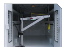
CORNER MOUNTED CARGO CRANE
